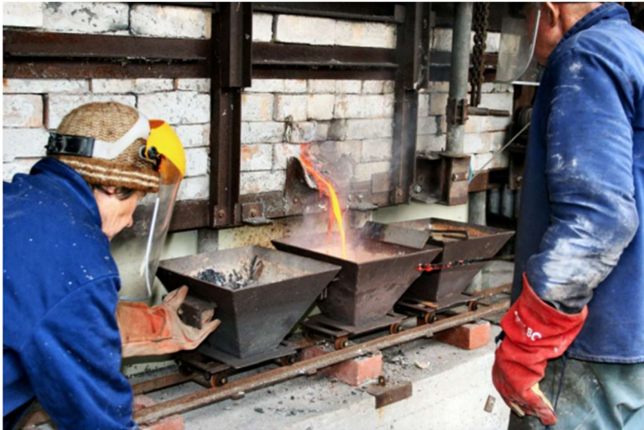
Tapping the furnace to release the molten tin.
