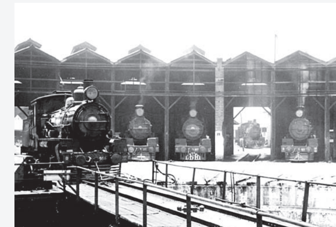
A locomotive approaching the turntable for spotting into one of the bays c1968
