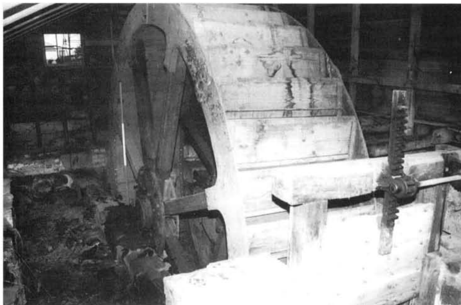
Fig. 4: Breastshot water wheel supplying power to Connorville Mill. Water is admitted into the buckets of the wheel through the sluiceway at right foreground. Range pole divisions are 50 centimetres (Photo W. Pearson, July 1993).
