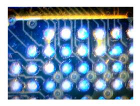
...the X-, Y-, and Theta axes micrometer adjustments can then be used to align the component and board (as shown at left). Once the component leads and pads are aligned, precise placement is ensured.
