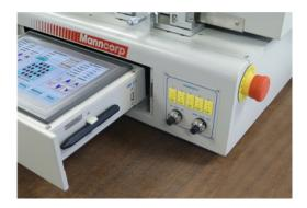
Touch Screen Control and Five Thermocouple Inputs for Precise Profiling
