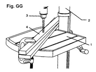
3. For small pieces that cannot be clamped to the table, use a drill press vise (optional accessory).
