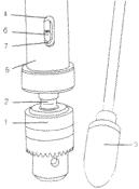
7. **(FIG. N)** Using a rubber mallet, plastic-tipped hammer, or a block of wood and a hammer, firmly tap the chuck upward into position on the spindle shaft.
