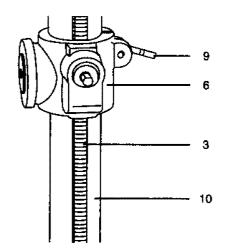
9. Install the collar (2) to the top end of the rack (3) on the column (10). Tighten the set screw (1).
