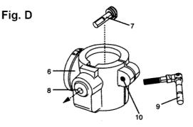
6. Place the rack (3) in position inside the table support (6), making sure the worm gear (7) on the inside of the table support is engaged with the teeth of the rack.
