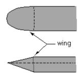
**Diagram 13.7 The wings on a spindle gouge**
