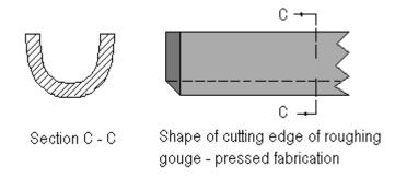
**Diagram 3.10 Shape of roughing gouge**
