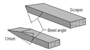
Diagram 3.3 Bevels on chisels and scrapers
