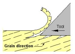
Diagram 7.4 Cutting against the grain Based on: Bruce Hoadley. (1980) Understanding Wood. Taunton Press
