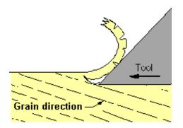
**Diagram 7.3 Cutting with the grain** Based on: Bruce Hoadley. (1980) Understanding Wood. Taunton Press
