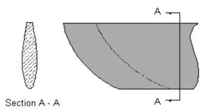
Diagram 3.5 Oval section HSS chisel with curved cutting edge
