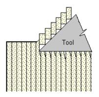
Diagram 7.5 Cutting end grain Based on: Bruce Hoadley. (1980) Understanding Wood. Taunton Press
