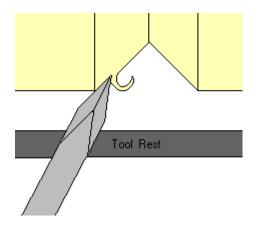
Diagram 12.10 The angle at which the tool is held for the push cut
