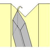
Diagram 12.9 The angle at which the tool is held for the swing cut
